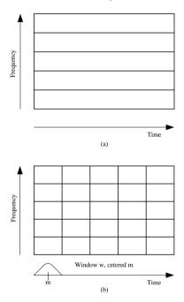
Figure 1. Comparison of the time-frequency plane (a) STFT and (b) Fourier transform.
